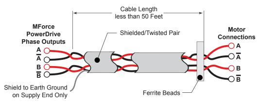
Figure 2.3.7: Motor Cabling Less than 50 Feet
